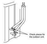
· Check the flare nut connections for the gas leak with a gas leak detector or soap water.
