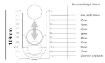
The Gel-clear APC19 is part of the bio-beta range of products for food retail refrigeration. A retrofit, adjustable pipe support for condensate drains running beneath chillers. Locks in place incremental slope settings. Statutory regulation requires a 19mm per metre slope on overground condensate drains.
